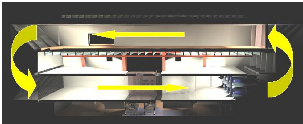
Figure 2: Longitudinal section showing the flow circuit; on the upper side is the boundary layer test section – on the lower side centre is the high speed low-turbulence test section – on the lower side at right is the 14 axial fans array
