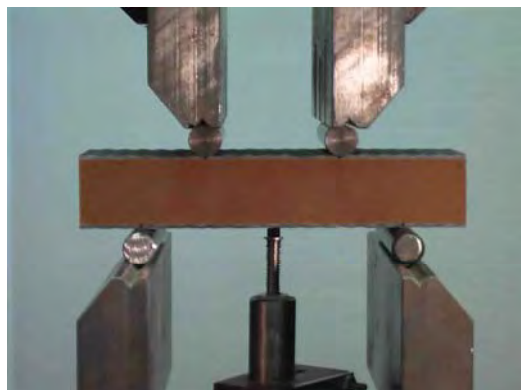
Figure 11: Short beam shear test setup
