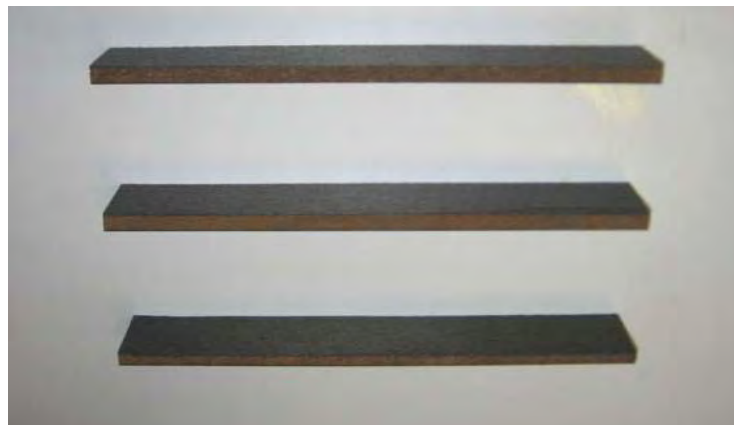
Figure 1: Cork agglomerate specimens
