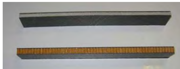
Figure 2: Rohacell and Honeycomb specimens
