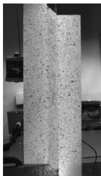
Figure 1: Block shear deformation of ductile core
