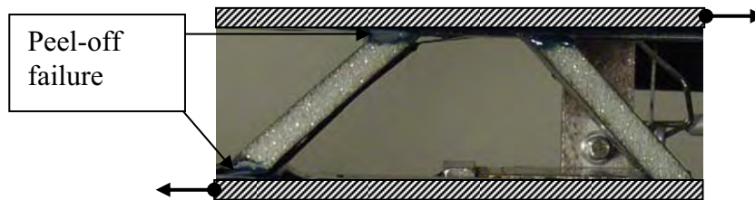
Figure 12: Shear testing of hierarchical 2 structure. The tensile loaded core member fails due to high peel-off stresses at the boundaries.
