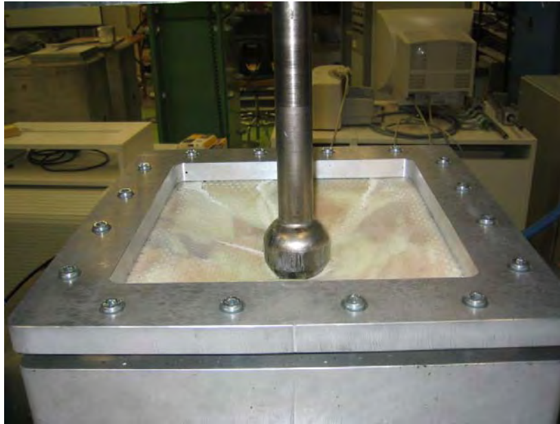
Fig. 3: Fixed support and the corresponding impactor for the perpendicular impact tests
