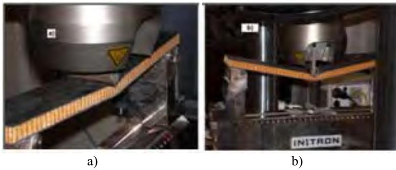
Figure 11: Failure sequence of the Honeycomb core specimens: a) Crushing of the facing in compression; b) core collapse
