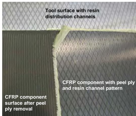
Figure 9: Tool integrated resin distribution system and component surface
