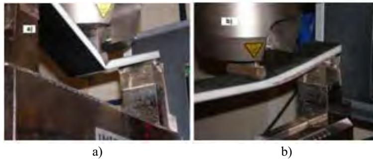
Figure 13: Rohacell modes of failure: a) core failure in the compression facing; b) facing debonding
