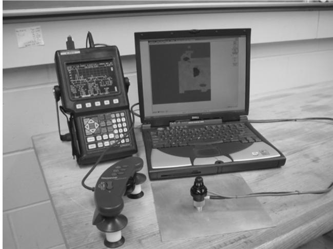
Figure 11. The Generic Scanner (“GenScan”) designed for generating C-scan images in the field.
