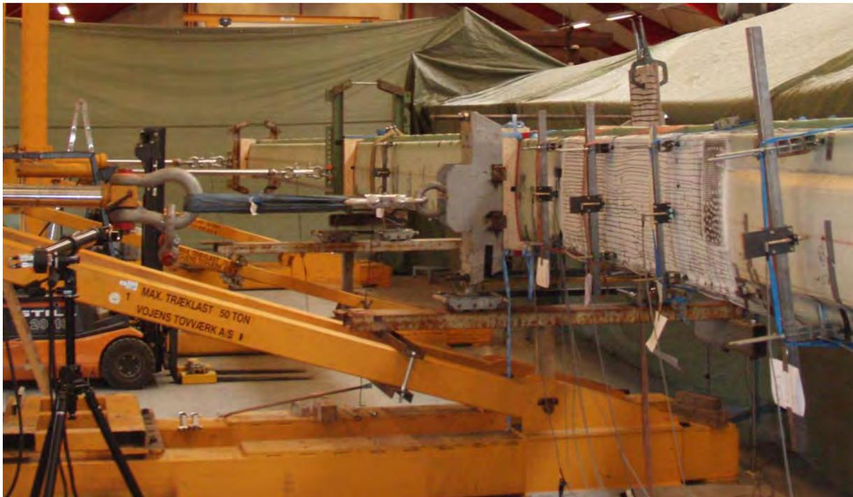
Figure 1: Full-scale test of load carrying box (box girder) from a 34m wind turbine blade
