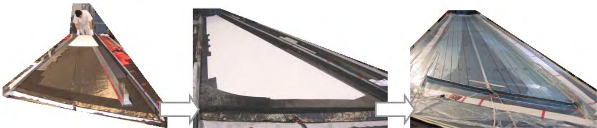
Figure 7: Large scale sandwich infusion demonstration (manual lay-up and infusion)
