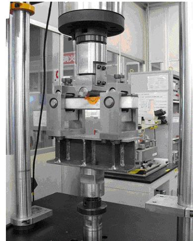
Fig. 7: Mode-II type test apparatus.
