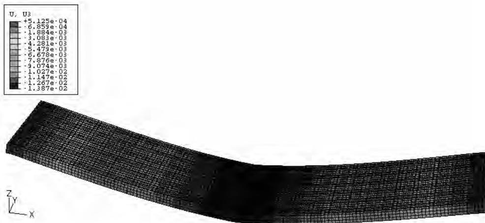
Figure 8: Deformation and displacement of long sandwich panel
