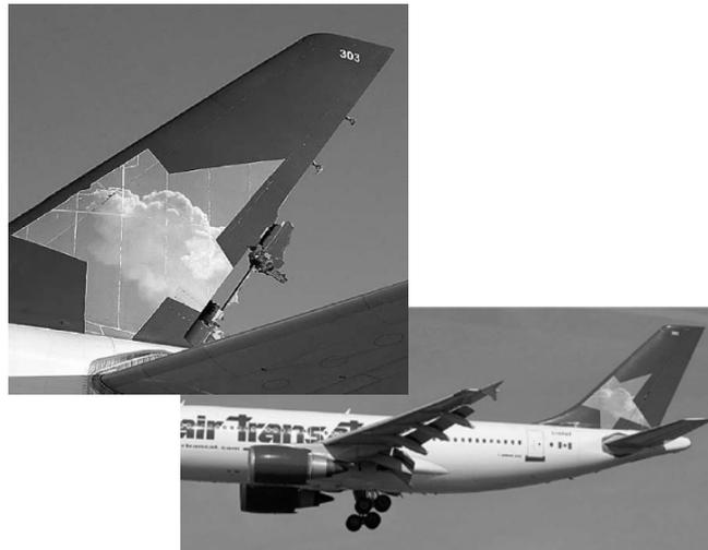
Figure 1. In-service failure of a critical composite sandwich structure in March, 2005.
