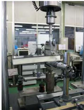
Fig. 6: Mode-I type test apparatus.
