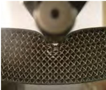
(a) Sandwich beam subjected to three-point bend loading
