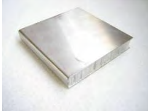
Picture 9: Steel skin glued on a nidaplast core
