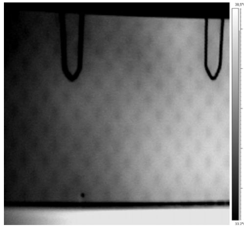
Figure 7: Infrared thermography image of welded Grid Sheet
