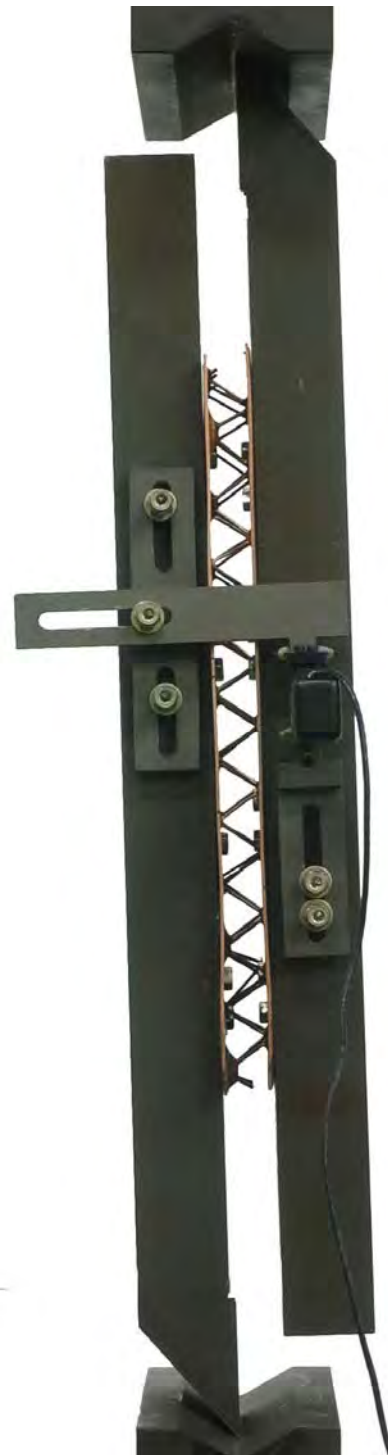
Figure 14 : Shear test specimen installed on grips
