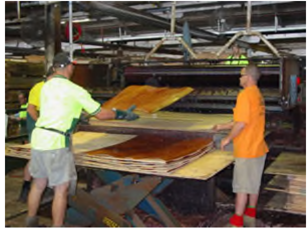
Veneer passing through the rollers of a glue spreader
