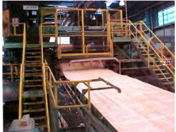
Veneer ribbon exiting lathe after peeling
