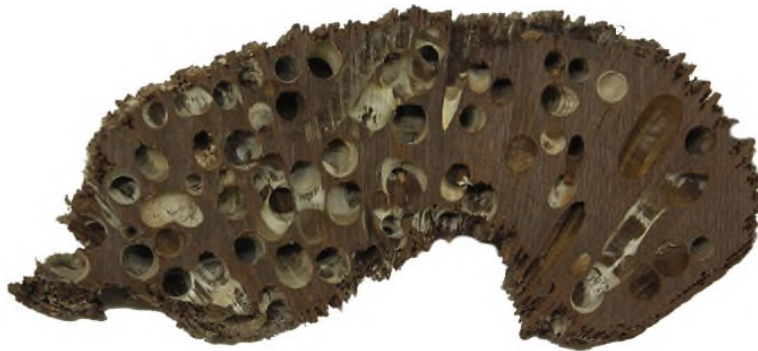
Marine borer damage to a hardwood pylon
